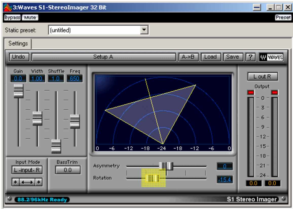
Figure 14 Stereo Imager - Correct any phase issues and RMS mismatches. If you have two different volumes for each track...DO NOT NORMALIZE to correct it. Just use the "Rotation" button while paying attention to the RMS levels in the "Level Meter"
