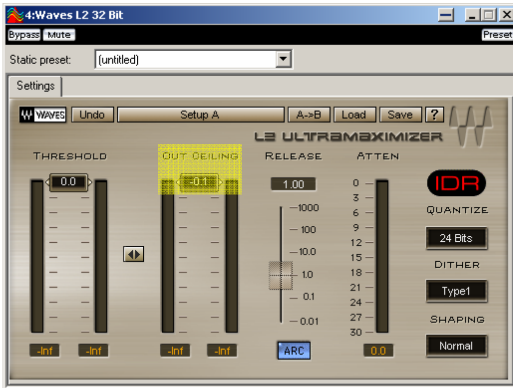
Figure 15 Limiter - Always use this and set the Out-Ceiling for -0.1. As you pull down the threshold fader slowly, look at the RMS level in your "Level Meter" If no longer see activity in your "out-ceiling" your song is too squished.
