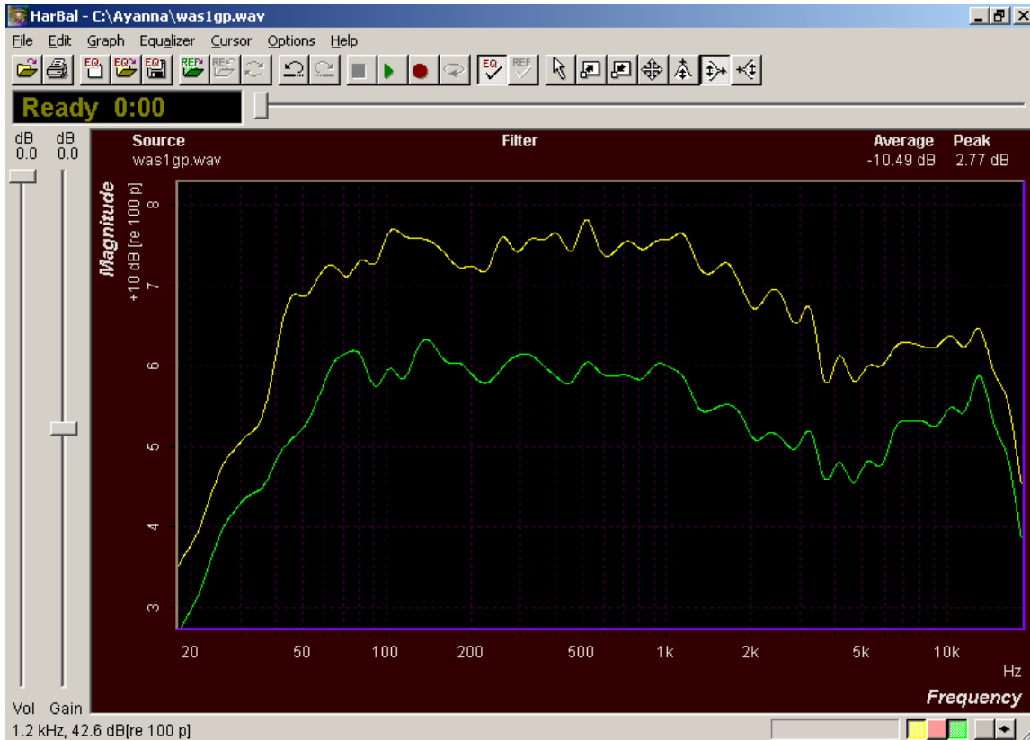
Figure 5 This is how your track should look before going any further. Do not worry about peaks to the right of the 5k mark. Getting rid of peaks (yellow line) and filling holes (green line) in the spectrum is the real magic of Har-Bal and prevents your compressor from working too hard.
