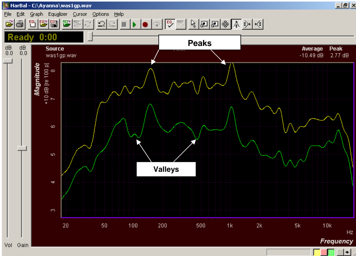
Figure 4 When you are finished mixing a track, import it into Har-Bal and check for peaks and valleys.
