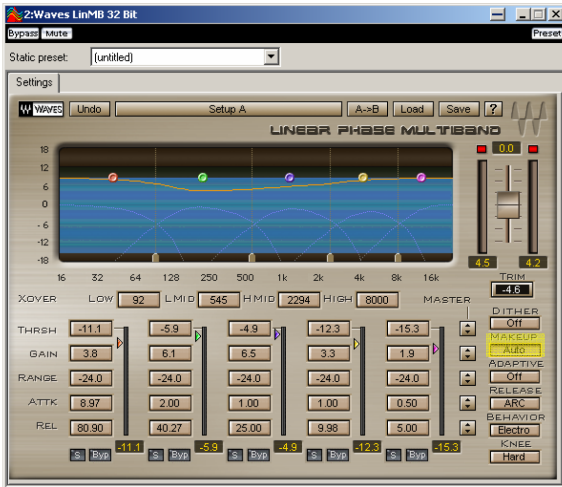
Figure 10 Click on the “Makeup” button on the right and change it to “Auto”. This will keep your volume the same while you are pulling down your master threshold.
