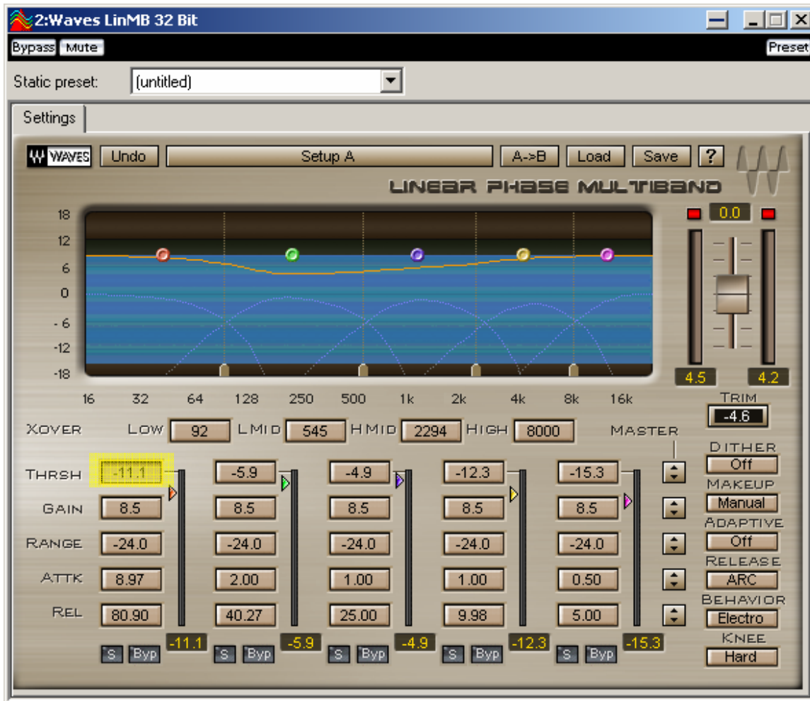
Figure 9 Change the threshold numbers for each band to match the new peak numbers that appear at the bottom.
